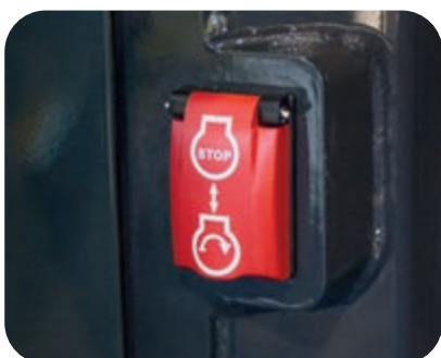
Secondary engine shutdown switch
