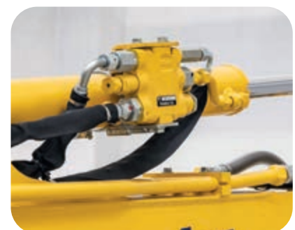
Hose burst valves on boom and arm cylinders
